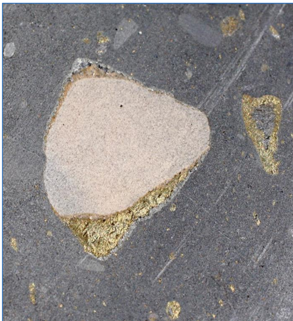
Figure 13.20 Typical Kamoa Hypogene Mineralisation in Diamictite
