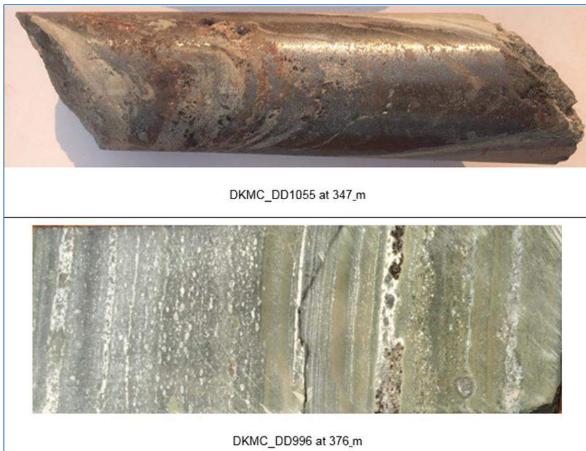
Figure 7.30 Examples of Coarse to Massive Chalcocite at Kakula
