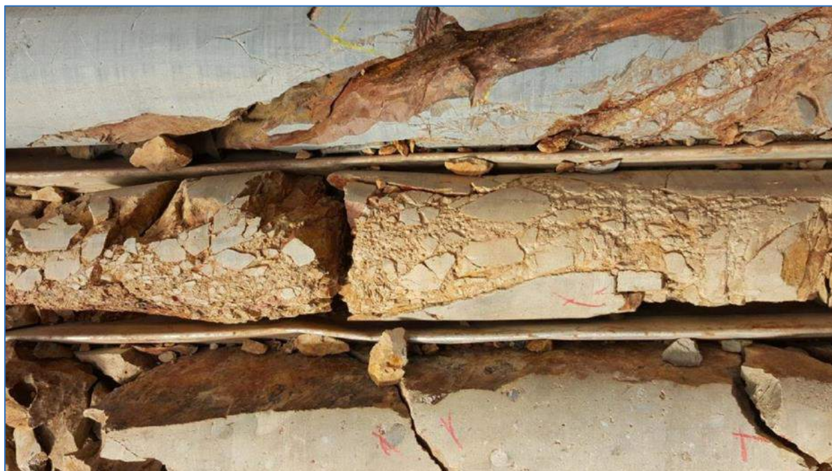
Figure 7.25 Steeply-Dipping Chaotic Breccia in DKMC_DD1015 (at 244.4 m)
