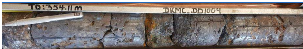
Figure 7.26 Massive Chalcocite Band Towards the Base of the Mineralised Zone in DKMC_DD1009 (at 354.1 m)
