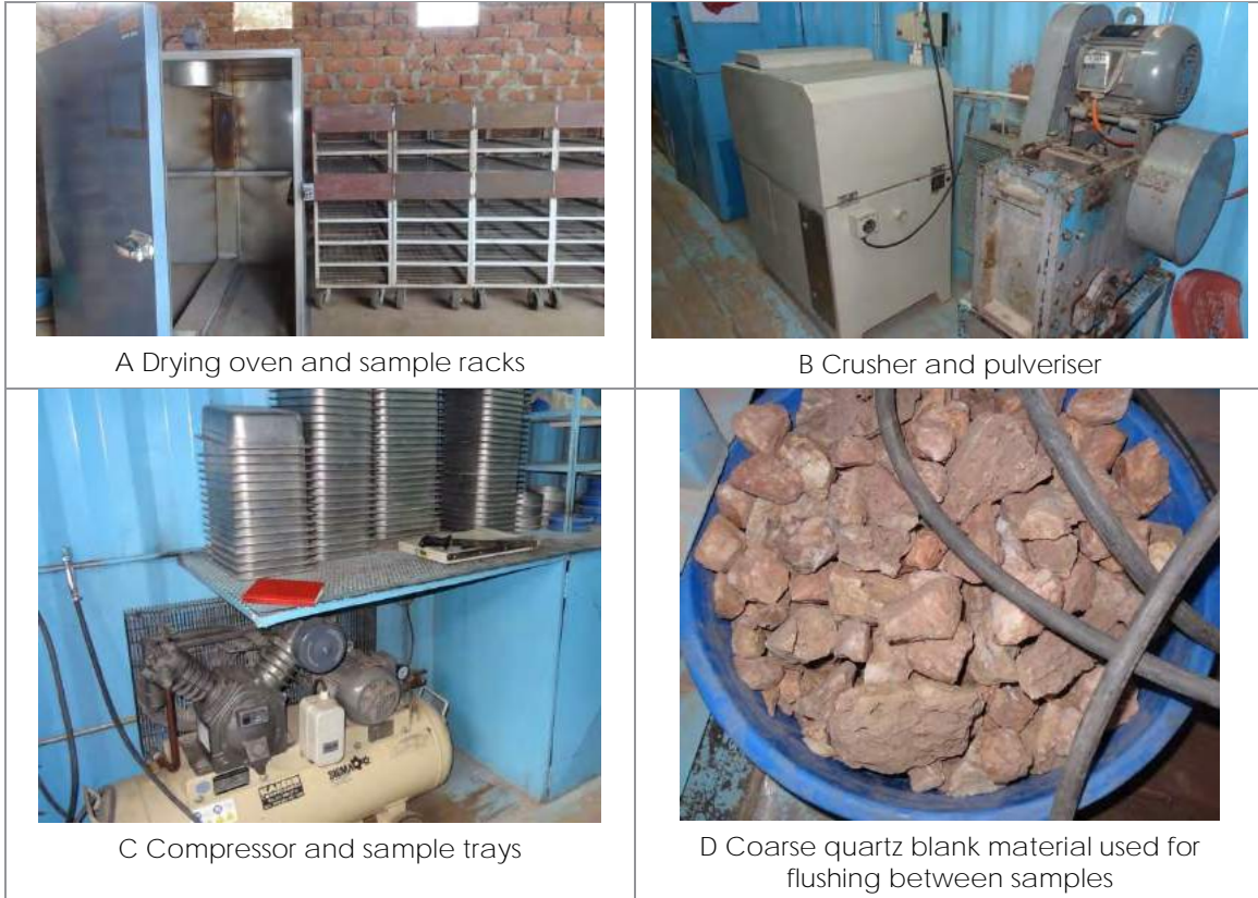
Figure 11.2 Containerised Sample Preparation Facility at the Kolwezi Laboratory
