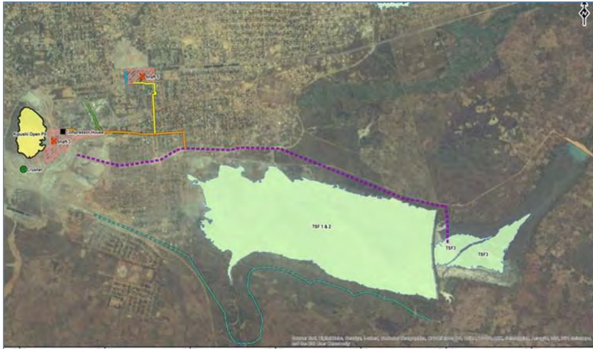
Figure 18.4 Kipushi Mine Drainage System
