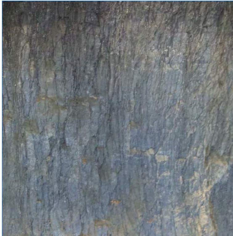
Figure 7.8 Incipient Development of an Anastomosing Spaced Cleavage in the Upper Kakotwe Formation Looking West on a Footwall Drive on -865 m Level. Foliation can be seen to Step Down-Stratigraphy (hence fabric steps down to the left in this photo)
