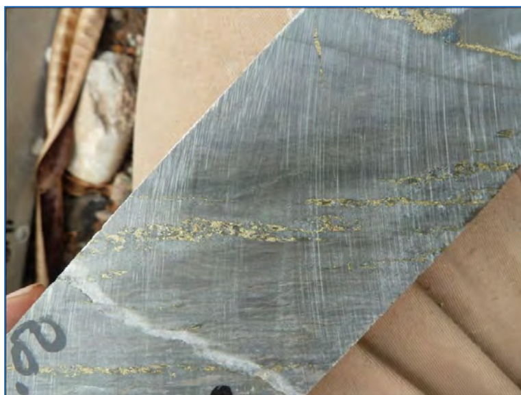
Figure 7.21 Blebby and Disseminated Chalcopyrite in Série Récurrente Siltstone at 148 m in Drillhole KPU074. Both Mineralization and Bedding are Deformed by Parasitic Folds
